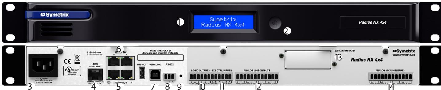
**1 Display:** Shows either an overview of system parameters or level meters for analog inputs, analog outputs, USB I/O, and expansion card I/O. The overview contains limited information such as IP Address, DHCP Status, and communication LEDs for Ethernet, Dante, and ARC. A short button press moves between the overview and input/output meters. The meters are scaled from -72 dBFS to 0 dBFS. Each segment represents 12 dB. If the signal reaches clipping, the meter will get wider.
