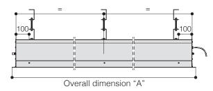
Width of the hole to be made in the false ceiling:  $\ensuremath{\textbf{22 cm}}$  .
