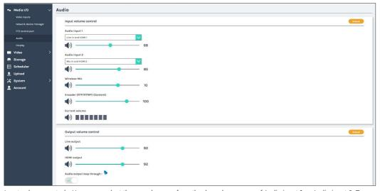
Input volume control - Users can select the sound source from the drop-down menu of Audio input 1 or Audio input 2. Tune the recorded volume from each audio input. Configurable range of sound input is 0-125,of AREC wireless microphone 0~15. The nearby volume meter indicates the encoded audio current volume.
