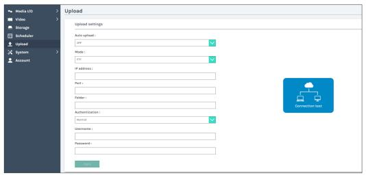
Auto upload- Select from the drop-down list. Start uploading "after recording is completed", or turn "OFF" the function. Followings to be configured according to the upload destination.
