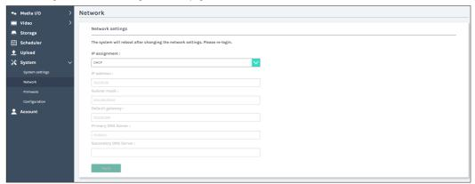
IP assignment – Select DHCP to have IP address be allocated by a router or any DHCP server being connected; or Select Static IP and enter the required network settings including IP address / subnet mask / default gateway/ DNS server.
