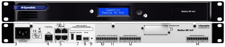
**1 Display:** Shows either an overview of system parameters or level meters for analog inputs, analog outputs, USB I/O, and expansion card I/O. The overview contains limited information such as IP Address, DHCP Status, and communication LEDs for Ethernet, Dante, and ARC. A short button press moves between the overview and input/output meters. The meters are scaled from -72 dBFS to 0 dBFS. Each segment represents 12 dB. If the signal reaches clipping, the meter will get wider.
