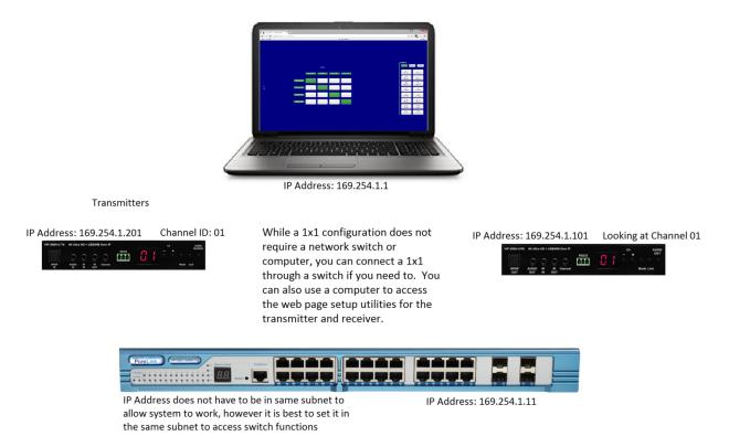
When the encoder and decoder are both factory set to Auto IP, they assign themselves unique IP addresses and therefore will work out of the box. The Channel ID must match on the encoder and decoder.
